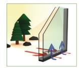
In the summer Super Spacer® minimises the heat exchange at the edges of the window panes and keeps the cool air indoors.
